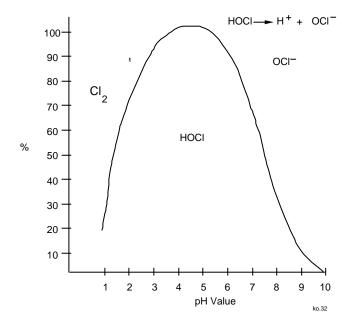
This chart shows that hypochlorous acid (HOCL) predominates between a pH of 3.0 and 7.0. Since corrosion increases as water pH is lowered, a pH of 6.5 to 7.0 is an optimum pH range for water contacting the metals found in most cooling water systems. Above a pH of 7.5, the less effective hypochlorite ion is the dominant species. HOCL formation is 50 percent at pH 7.5 and declines rapidly as pH increases.
