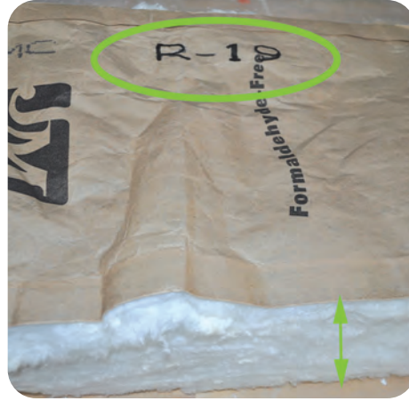
2. Insulation R-value matches work order
