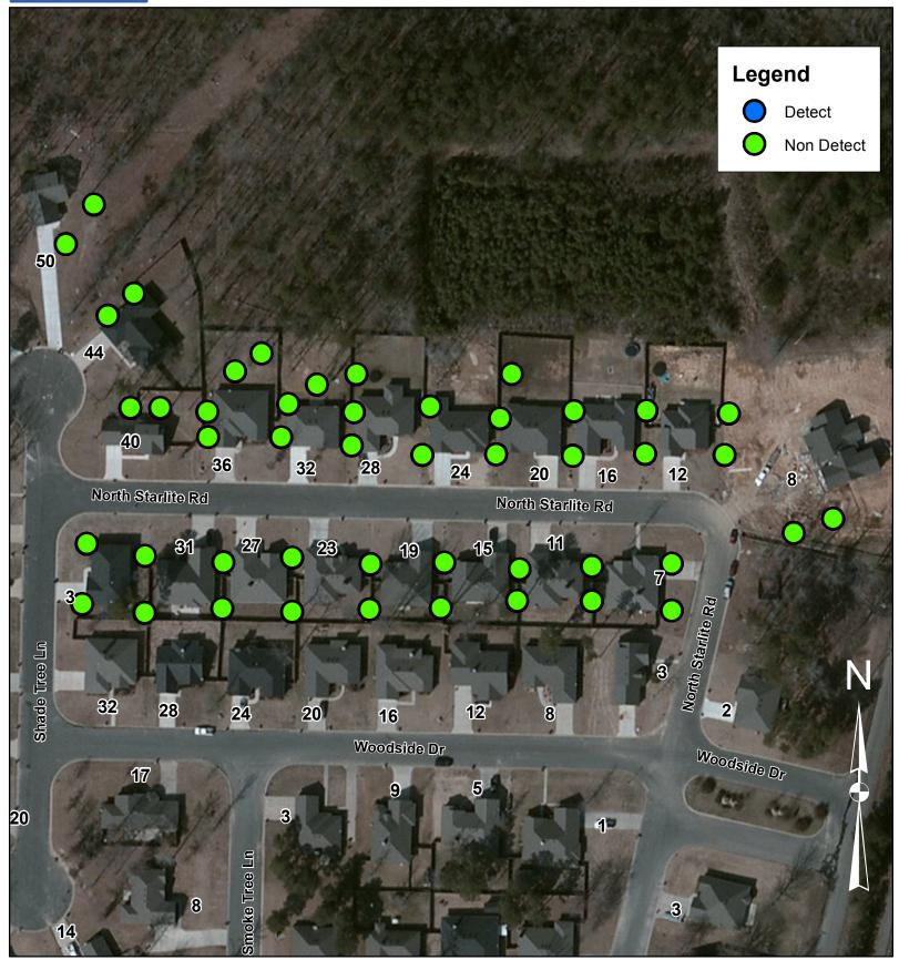
The above locations were monitored for Benzene, VOC, and H2S during the night shift. All readings were below the limit of detection for the instruments used.
