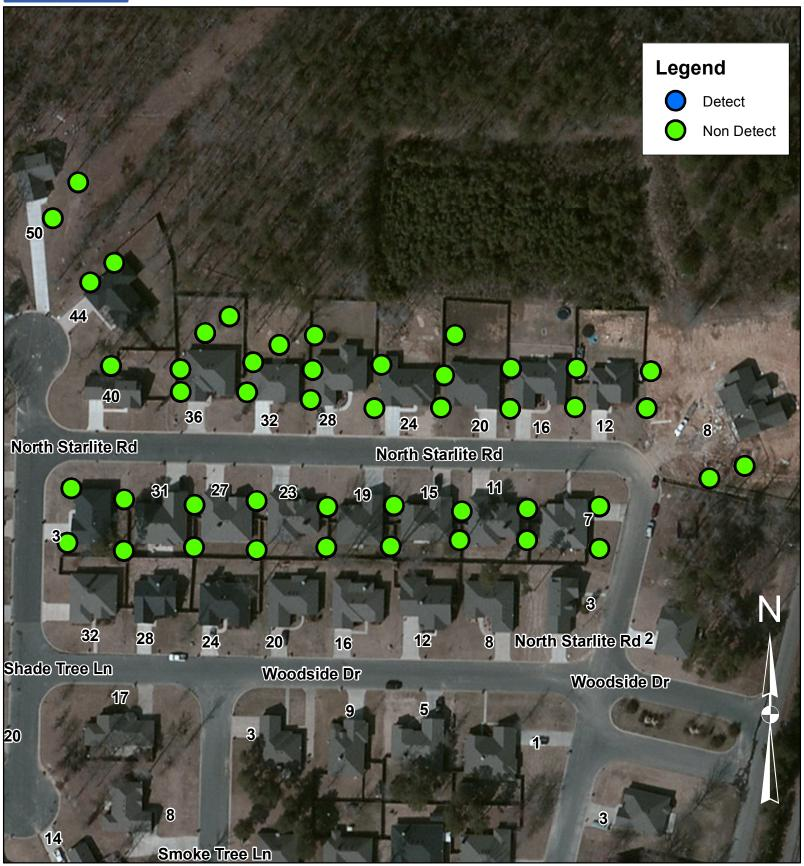
The above locations were monitored for Benzene, VOC, and H2S during the Day shift. All readings were below the limit of detection for the instruments used.
