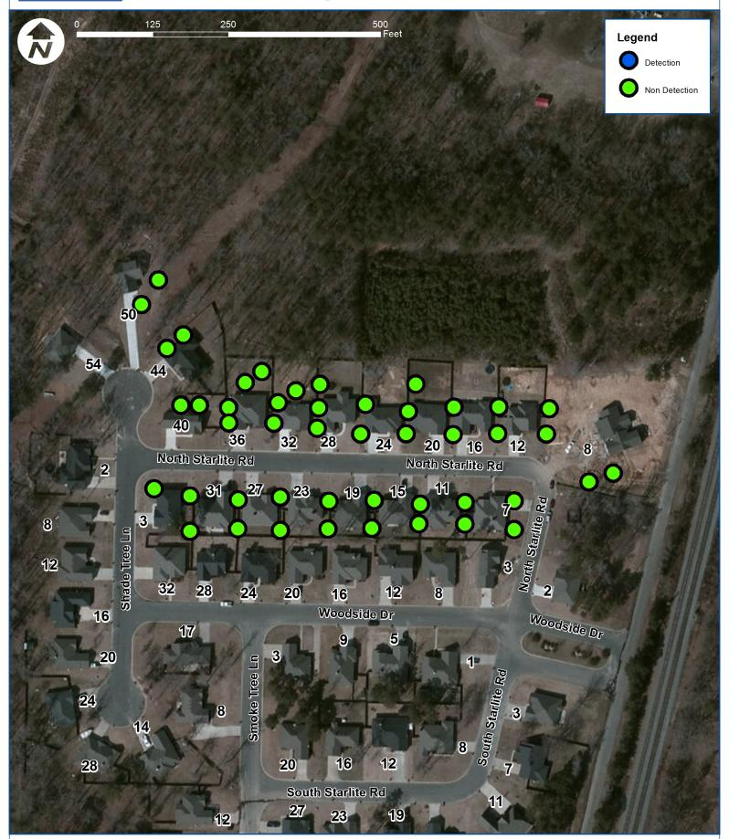
The above locations were monitored for Benzene, VOC, and H2S at the beginning of the night work shift 4/10/2013. All readings were below the limit of detection for the instruments used.
