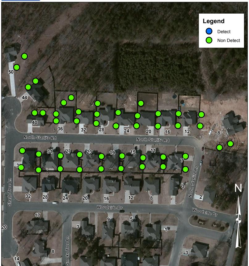
The above locations were monitored for Benzene, VOC, and H2S during the night work shift 4/13/2013. All readings were below the limit of detection for the instruments used.
