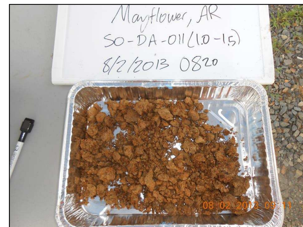
1.0 – 1.5 ft SILTY CLAY/CLAYEY SILT (CL/ML), low plasticity, dry, soft, light brown, no odor, no organics
