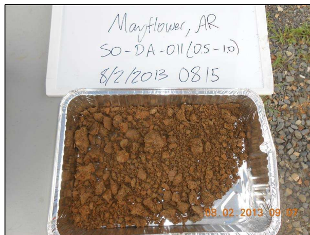
0.5 – 1.0 ft CLAYEY SILT (ML), no plasticity, dry, soft, brown/reddish brown, no odor, trace organics
