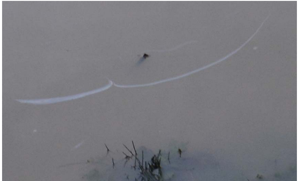
Non-Brittle Sheen Picture – Without a Polarizing Filter
