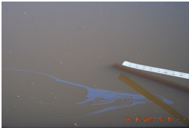
Silver Gray Sheen Patch/Streamer Observation with an Oil Spot (0.125-inch Wide) on 07/16/2015
