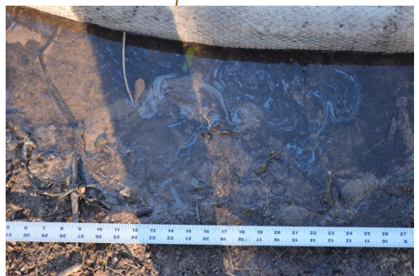
Rainbow Sheen Streamer with Small Oil Spots (0.1-inch Wide) Observation on 01/02/2014
