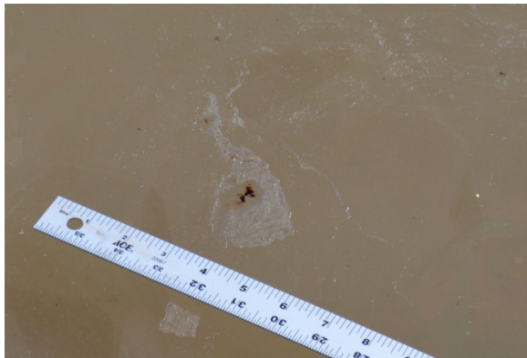
Rainbow Sheen Streamer with Small Oil Spot (0.25-inch Wide) Observation on 12/31/2013
