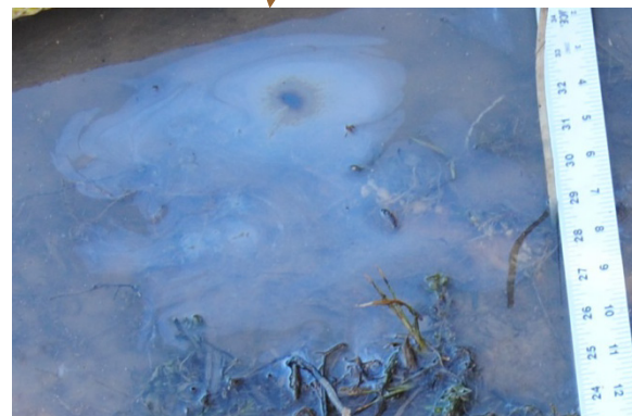
Rainbow Sheen Patch with Oil Spot (0.75-inch Wide) Observation on 01/16/2014
