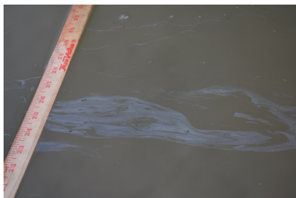
Dark/Metallic/Rainbow Sheen Streamer with Oil Spots (0.1-inch Wide) on 01/14/2014
