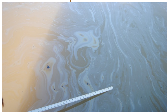
Silver Gray Sheen Patch/Streamer with Oil Spot (0.1- to 0.75-inch Wide) Observation on 01/20/2014
