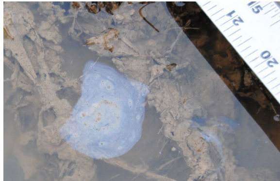
Silver Gray Sheen Patch with Oil Spots (0.5-inch wide) Observation on 03/02/2014
