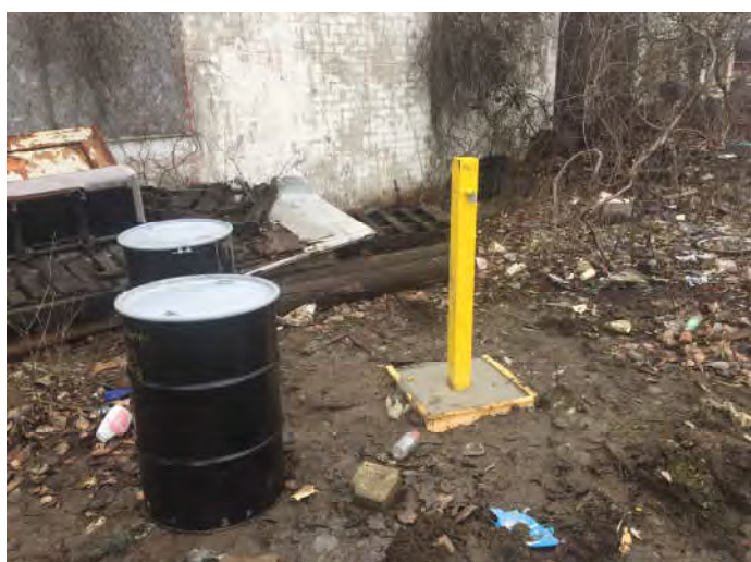
Photo 5. Above-ground stick-up completion, MW-3.
