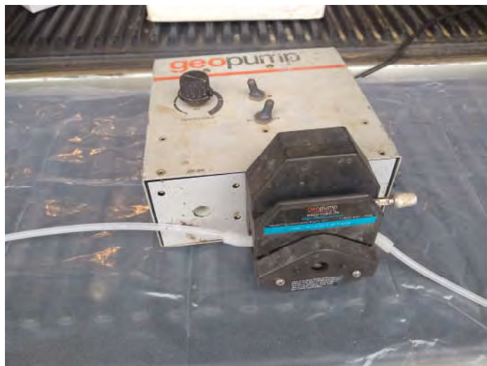
Photo 9. Peristaltic pump used for groundwater sampling.
