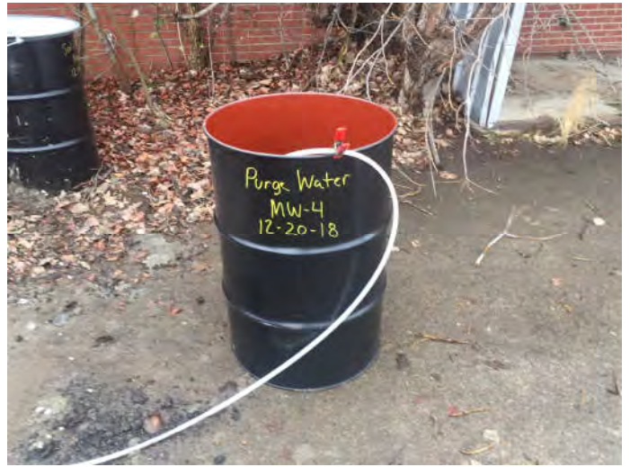
Photo 8. Well development discharge into 55-gallon drum.
