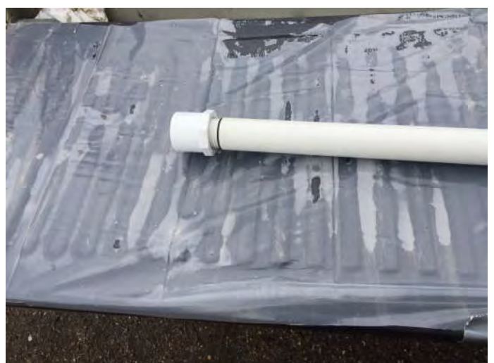
Photo 6. Surge block used for well development.
