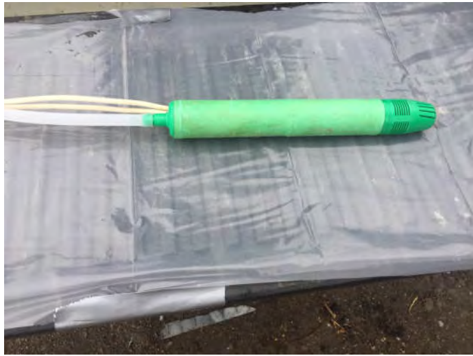
Photo 7. Submersible pump used for well development.
