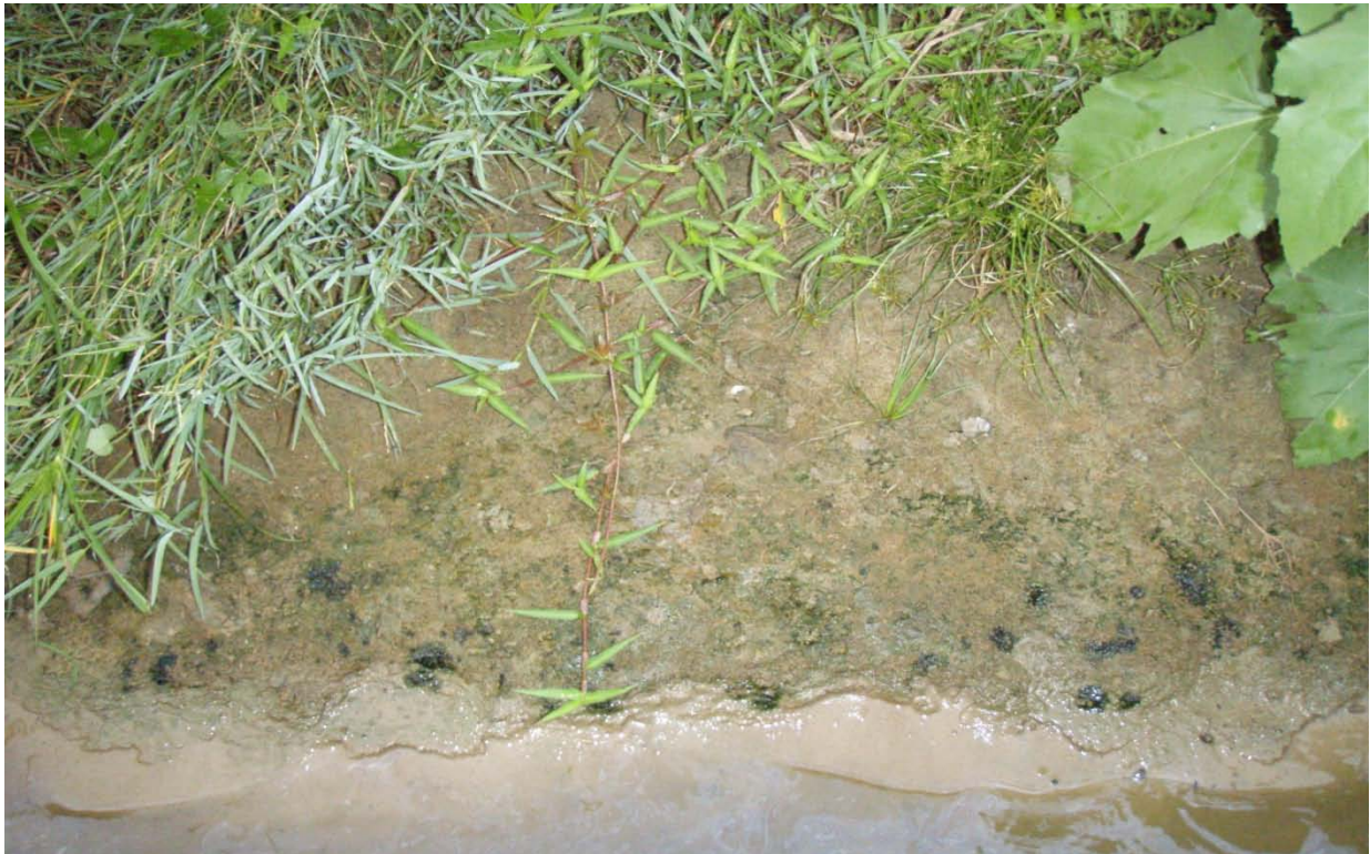
Figure 4.19. Study Reach LC-1 during low flow conditions. Recently deposited stream bank sediments. Note dark globules in sediment. The dark spheres are oil/tar sediment masses. August 2010.
