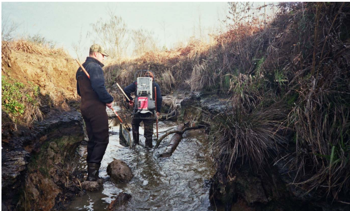
Figure 4.26. Study Reach LC-3. View to upstream. Electroshocking to characterize the fish community. Note the hydrocarbon laden soil layering on left and right banks about 3.5 feet above water surface. January 2009.
