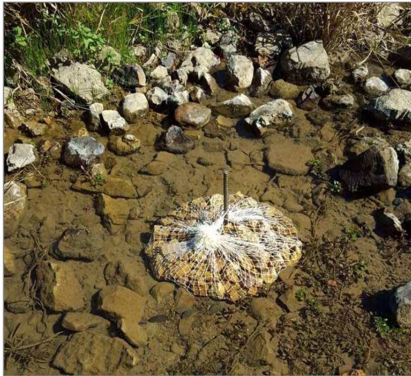
Figure 2.6. Photograph of newly deployed rock bag sampler.
