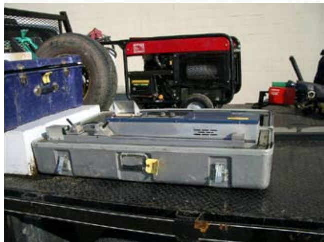
Figure 10E-22 Field tensiometer (Source: Poly-Flex, Inc., 1995)
