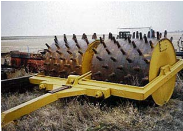
Figure 10D-19 Modern type of tamping roller less well suited for compacting soils for clay liner
