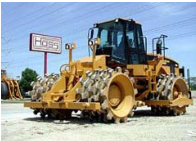
Figure 10D-19 Modern type of tamping roller less well suited for compacting soils for clay liner
