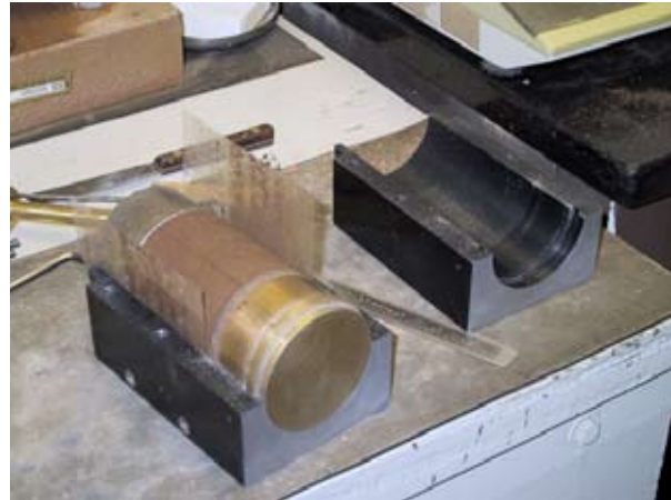
Disassembled mold with compacted specimen
