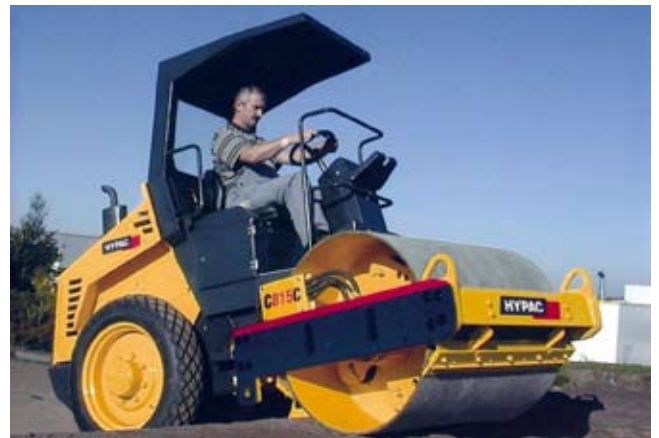
Figure 10D-20 Smooth-wheeled steel roller compactor
