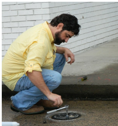
An ADEQ geologist prepares to sample a monitoring well at a Pulaski County service station where gasoline leaked from an underground storage tank.
